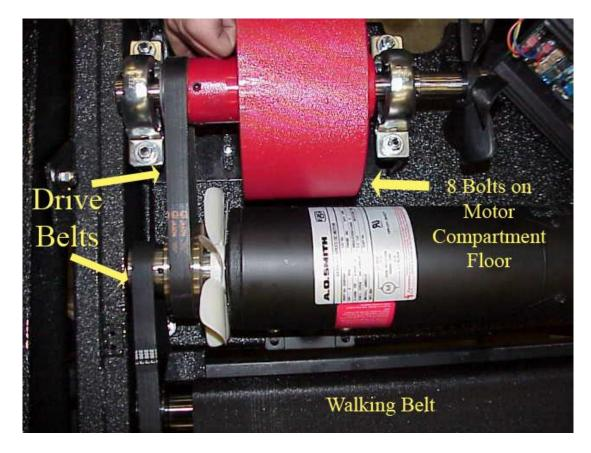
There are two steps in adjusting the drive belts after a belt or motor replacement: Step 1: Tighten the motor belt and bolt the motor down to lock it into position. Step 2: Loosen the flywheel belt and bolt the flywheel down to lock it into position.
