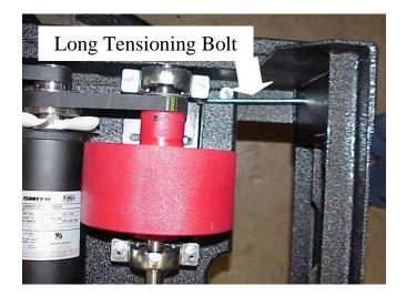
Use a <sup>1</sup>/<sub>2</sub>" socket wrench to tighten the tensioning bolt just enough to remove the belt slipping. Check the tension on the belt that runs from the motor to the front roller by twisting or wiggling it. You should be able to twist the belt about 90 degrees.
