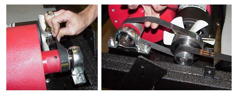
When the flywheel belt has been loosened to the correct tension, tighten the four bolts that hold the flywheel to the floor of the motor compartment.
