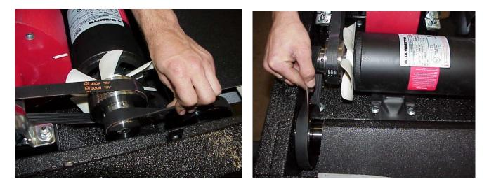
If you wiggle the belt up and down, there should be at least  $\frac{1}{2}$ " of play. Be careful not to over-tighten the motor belt. **Over-tightening the motor belt will cause the motor shaft to snap and void the warranty.**
